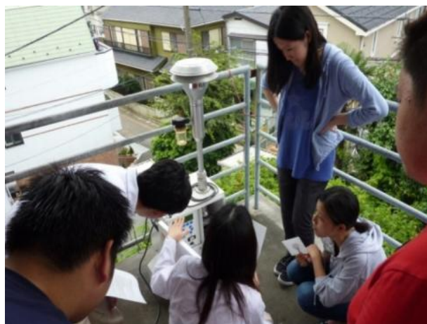
Fig.1 Sampling of PM 2.5 by high school students at central Tokyo (July 2013 ~ May 2014)
